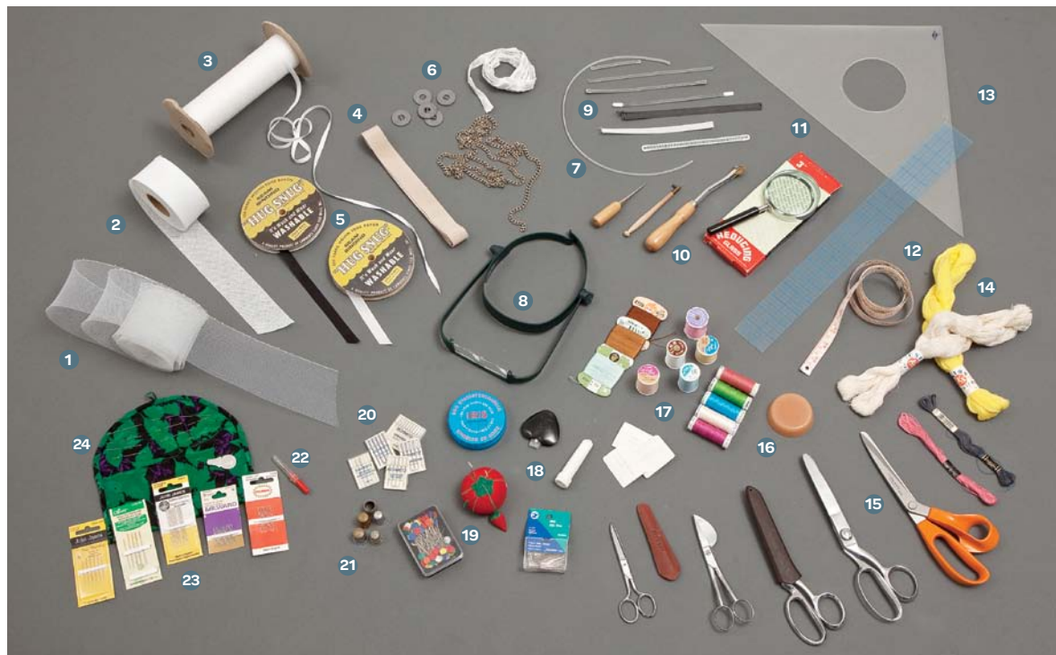
Horsehair braid (1), wigan (2), stay tape (3), Petersham (4), seam binding (5), weights (6), spiral boning (7), magnifier (8), boning stays (9), tracing wheel (10), reducing glass (11), measuring and drafting equipment (12), homemade pouncer triangle (13), basting cotton (14), scissors (15), beeswax (16), thread (17), chalk (18), pins (19), machine needles (20), thimbles (21), tambour hooks (22), needles (23), silk pin bag (24). (Photo by Taylor Sherrill. Author's collection.)
